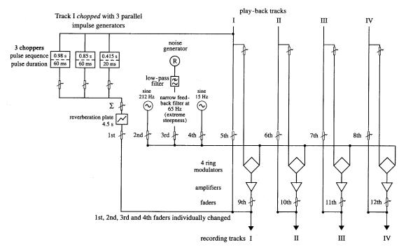
The 3 chopper outputs were controlled as equally important, in order to maintain the irregular rhythm without dominating periods. The output of the reverberation plate with 4.5 seconds reverberation was connected to track I.
